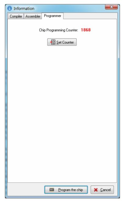
Pressing the Set Counter button will open the Set Programming Counter window:
